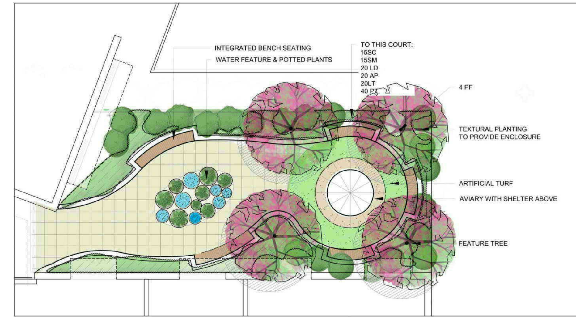
1b LEVEL 1 DEMENTIA COURTYARD - EAST SCALE 1:100
